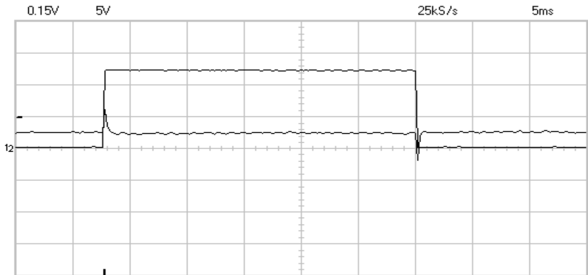
Fig. 11. The signals from the power switch's gate (upper) and comparator input (lower). The comparator output and "Reset" input of RS-trigger are disconnected (i.e. the circuit generates 30 ms pulse). The reaction to front and back of this pulse, and the noise signal are clearly visible.
