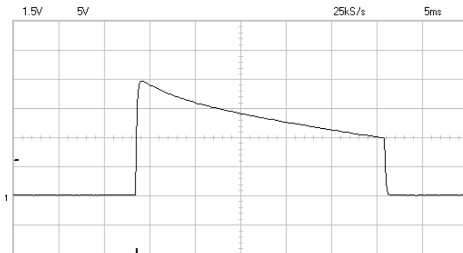
Fig. 7. Voltage on CS resistor (no projectile). Scale on vertical axis – 1.5 V/div (thus, maximum current is about 60 A).
